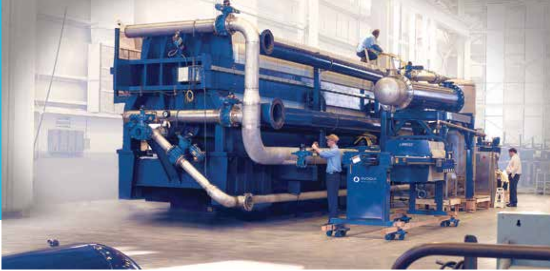
The J-Press® filter press can be configured with highly sophisticated manifolds, controls and cake discharge systems, such as this 2.0 m x 2.0 m J-Press® filter press built for a prominent municipal wastewater treatment plant.
